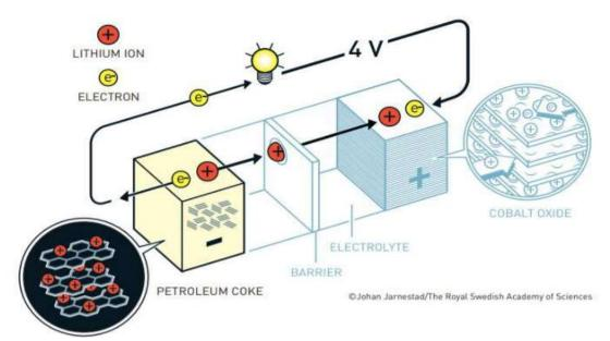
The advantage of lithium-ion batteries is that the chemical current produced in them is based on the movement of lithium ions flowing between the anode and cathode, rather than a chemical reaction that ends with the breakdown of the electrode.
