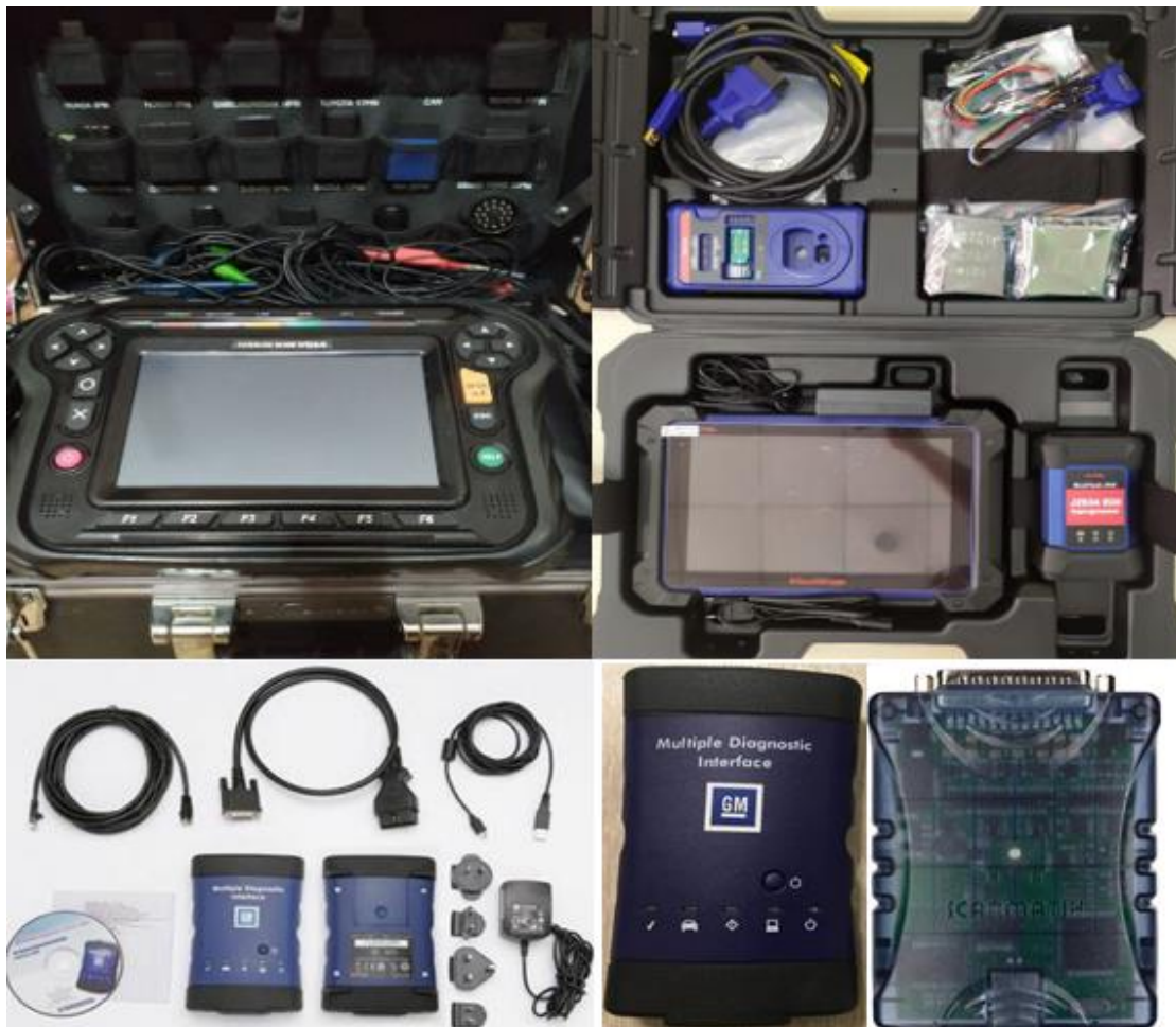
Figure 4. Diagnostic and measuring equipment used in this work for reading and calibrating mechatronic control systems of the engine and the vehicle [8].
