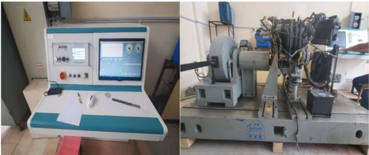
Figure 3. Hardware-software complex for the experimental determination of the dynamic characteristics of the internal combustion engine
