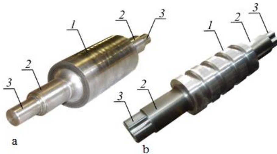
Figure 1. Integrated worker bees: a - smooth; b - profiled; 1 - barrel; 2 - neck; 3-running tips
