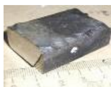
Figure 1: Samples taken from the working parts of Stone Crushers
