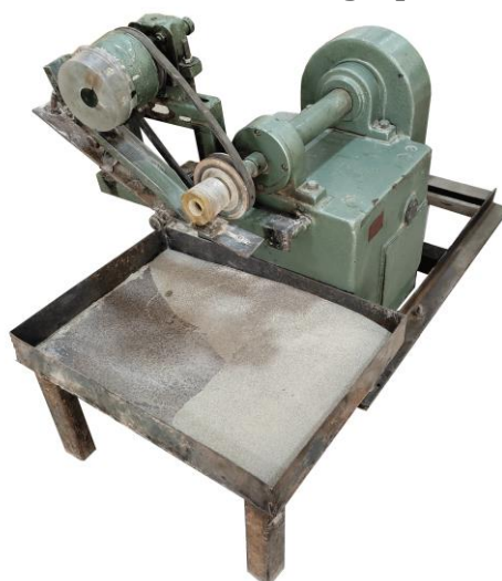
Figure 5: Device for testing samples for abrasive wear.
