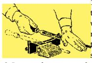
1. The rough product is planned. It is clamped in such a way that the concave part is at the top. The concave surface is smoothed with the rounded part of the semi-circular groove, leaving 0.1-0.2 mm; During operation, the device is slightly turned and moved to the right or left along the surface being treated. The concave surface is processed along longitudinal lines.
