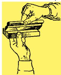
Dirt on the treated surface is removed with a brush or cloth. The material is removed from the gira, and its wide surface is treated in any of the previously indicated ways (longitudinal, transverse or cross lines). After 1-2 passes, the material is removed from the machine and the quality of the surface is checked with a level ruler as follows:
