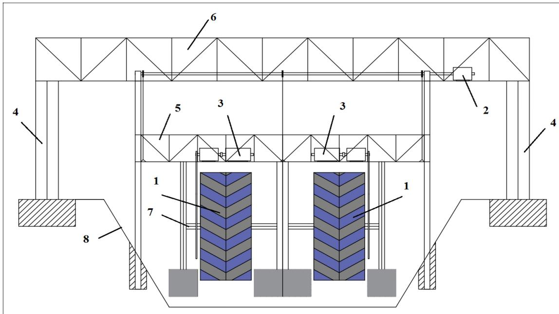
**Figure 4. Micro HPP scheme proposed by the author: 1-wheel impeller (diameter 2 meters), 2-engine moving the wheel up and down, 3- generators, 4-supports, 5,6 farm, 7-wheel axle, 8 - the source.**
