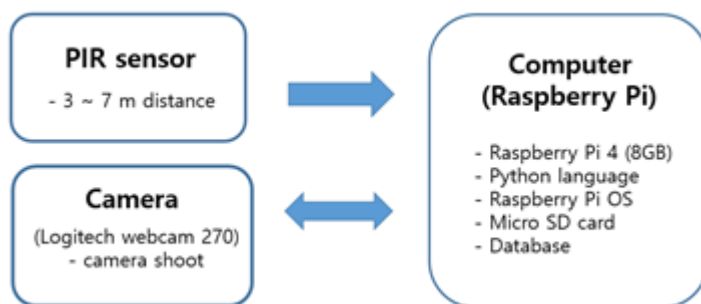
Figure 7. The configuration diagram of the Smart Home Security System
