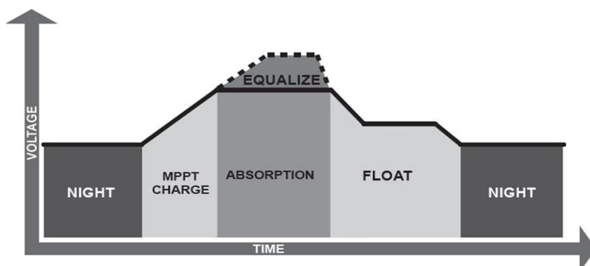
Figure 1. Optimal charging algorithm
